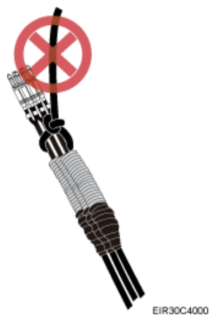
Figure 7-8 Incorrect binding method
