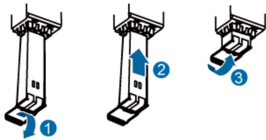
Figure 9-24 Installing an optical module
