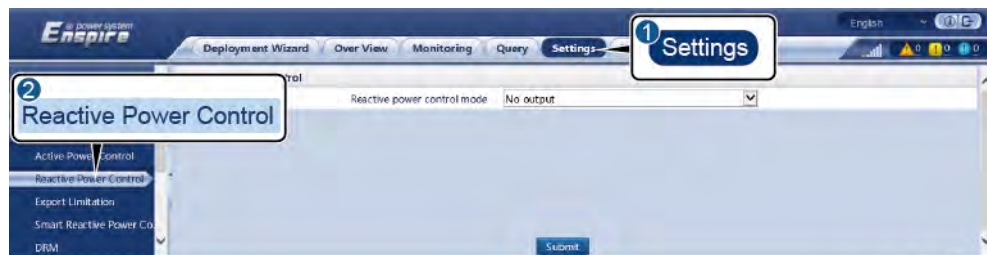
Figure 6-43 Reactive power control
