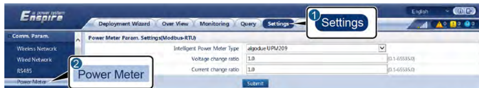
Figure 6-24 Setting power meter parameters
