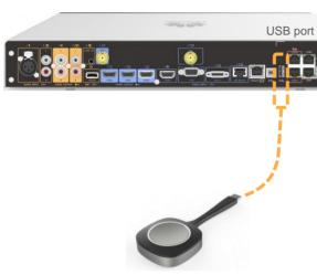
Pair an AirPresence Key with the Box when they are used together for the first time. HUAWEI Box 700 is used as an example.
