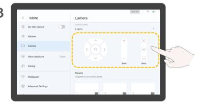
Tap arrow keys, +, -,  $\begin{bmatrix} + \end{bmatrix}$  ,  $\begin{bmatrix} - \end{bmatrix}$  , and  $\begin{bmatrix} AF \end{bmatrix}$  to adjust the camera.
