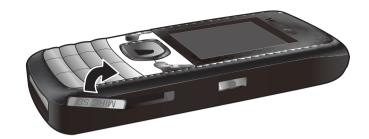
To remove a memory card, open the rubber cap and press the memory card gently. Now the memory card will pop up automatically. Then take it out as shown in the following figure.
