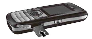
2 After inserting the memory card completely, replace the rubber cap.
