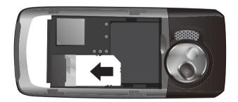
To remove the SIM card, power off your phone and take out the battery. Then press the SIM card with one finger and slide it out of the slot.
