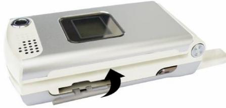
3. To remove a memory card, open the rubber cap and press the memory card gently. Now the memory card will pop up automatically. Then take it out as shown in the following figure.
