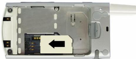
3. Slide the USIM card into the card slot as shown in the following figure.
