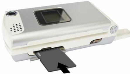
2. After inserting the memory card completely, put on the rubber cap again.
