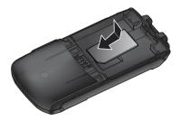
2 Fit the battery into the battery slot on back of the phone. Press the battery down until it clicks into place.
