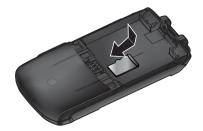
To remove a memory card, power off the phone and remove the battery. Then press the memory card gently. Now the memory card will pop up automatically. Then take it out as shown in the following figure.
