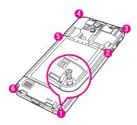
Use tweezers to lever the rear housing up, following the sequence as shown in the following figure. Avoid excessive force in order to not accidently bend the rear housing.
