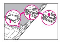
**Caution:** Gently remove the battery connector to prevent damage to the connector.
