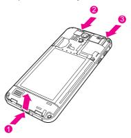
4. Remove the battery connector.
