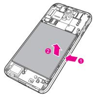
Caution: The Li-polymer battery is packed with a soft material. Do not use a sharp tool to lever the battery out because doing so may result in damage to the battery. Damaging the battery packaging material could result in spill of highly combustable or toxic chemicals which may constitute a fire hazard or could be damaging to your health. Therefore, it is recommended that you gently use the blunt end of the tweezers to lever the battery out.
