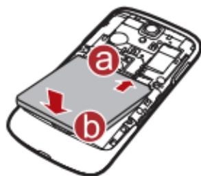
1. Angle the edge labeled **a** (with the contacts) into the bottom end of the battery compartment.
