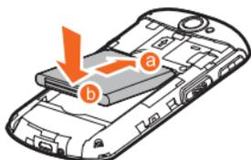
1. Angle the edge labeled **a** (with the contacts) into the bottom end of the battery slot.
