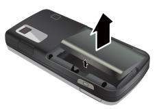
**3** Press the SIM card with one finger and slide it out of the slot.
