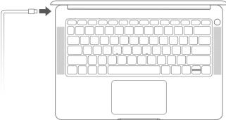
Your MateBook is pre-installed with an irremovable, rechargeable battery. You can charge your MateBook with the adapter and USB-C charging cable that comes with it. The battery is sufficiently charged when the charging indicator stays steady white.
