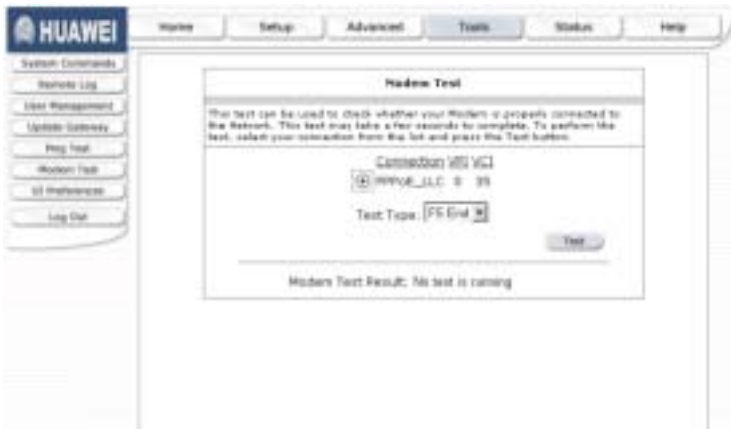
Figure 3-45 Tools – Modem Test window
