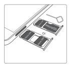
The upper card slot may not support nano-SIM cards. You can insert only a microSD card into it.
