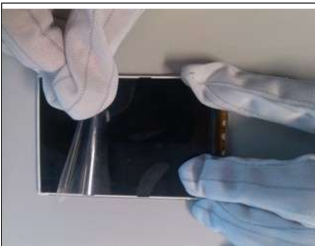
6. Remove the protective film from the LCD.
