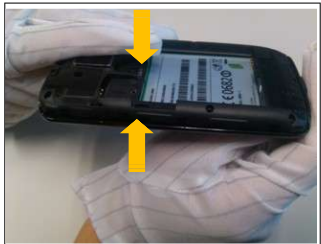
13. Install cover B: Snap cover B's bottom, and press its top.
