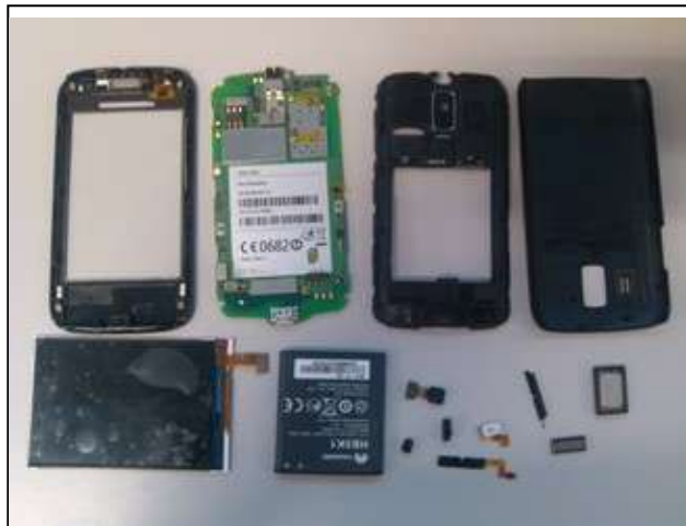
21. The phone is now disassembled.
