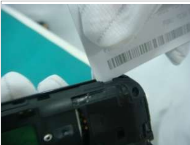
6. Use the disassembly tab to release the latch in the upper left corner.
