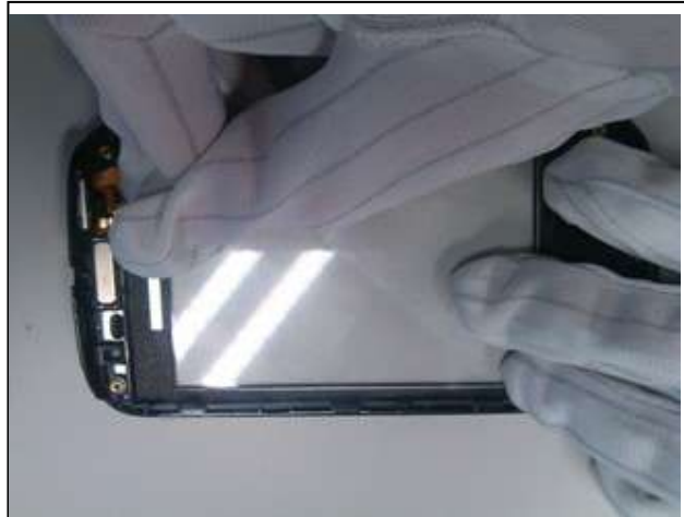
5. Remove the protective film from the touchscreen panel.
