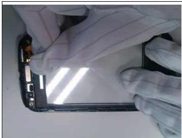
17. Apply a protective film on the inner side of the touchscreen panel.
