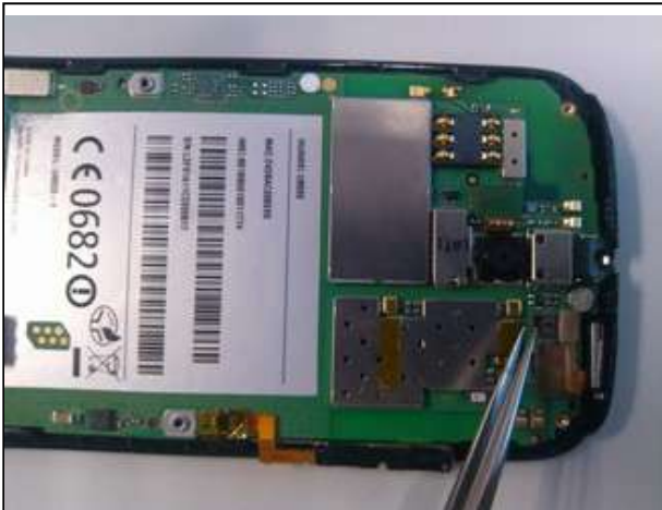
10. Disconnect the BTB connector cable between the touchscreen panel and the LCD.
