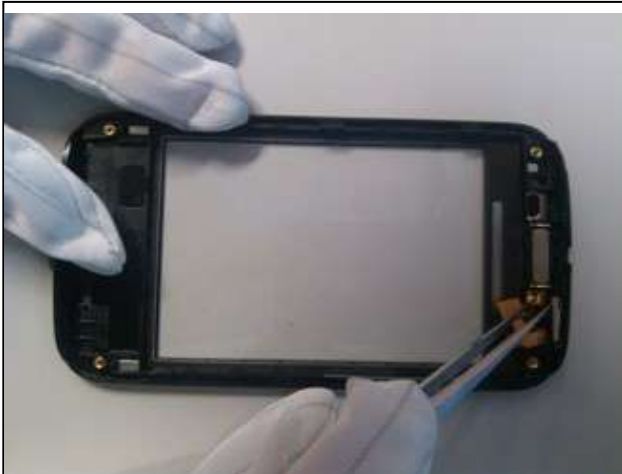
4. Install the Power key FPC.
