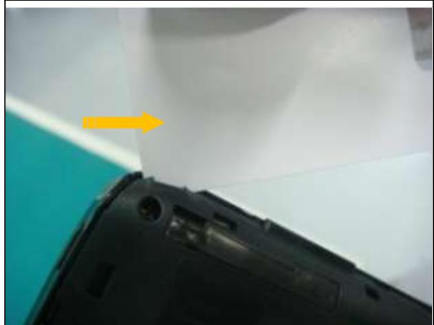
5. Use the disassembly tab to release the latch in the upper right corner.
