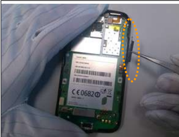
8. Remove the volume key.
