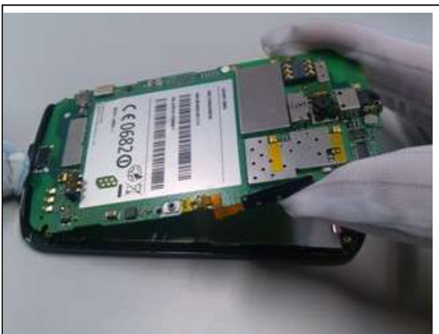
8. Install the PCBA: Insert the USB port into cover A, and then snap the PCBA downward in place.
