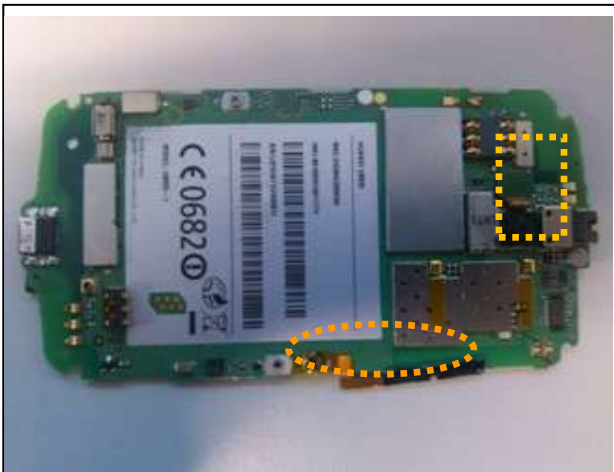
14. Release the BTB connector, and remove the camera. Release the ZIF connector, and remove the volume key FPC.
