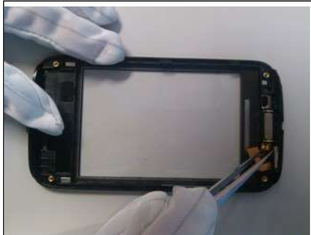
19. Remove the receiver.
