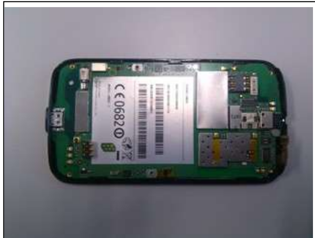
11. Release the two latches in the PCBA.
