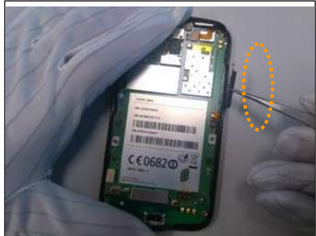
11. Install the volume key: Attach the volume key FPC to the metal piece on cover A, and then install the volume key.
