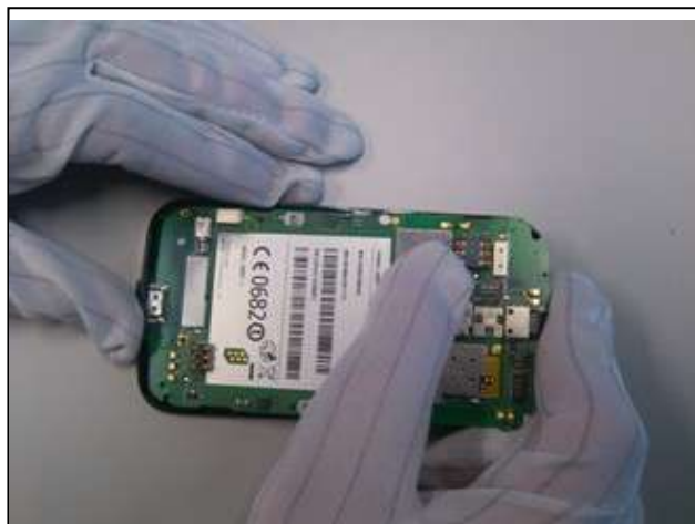
9. Gently press the PCBA to close the latches to secure the PCBA.
