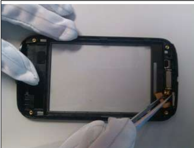
18. Remove the Power key FPC.
