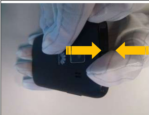
16. Install the battery cover.
