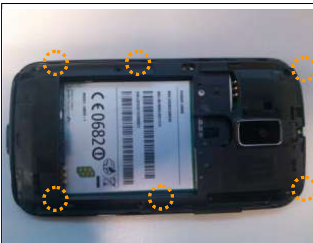
14. Install the six screws into cover B.
