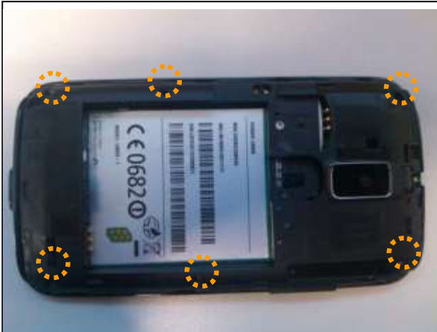
4. Remove the six screws from cover B.
