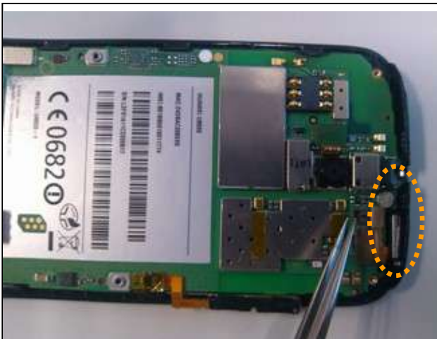
10. Snap the LCD's BTB connector and then the touchscreen panel's BTB connector in place.
