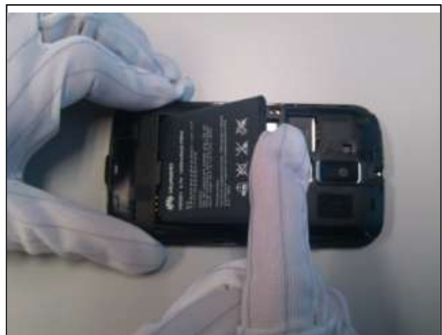
15. Install the battery: Insert it into the battery compartment bottom first.
