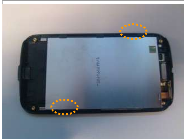
15. Release the LCD latches, and remove the LCD.
