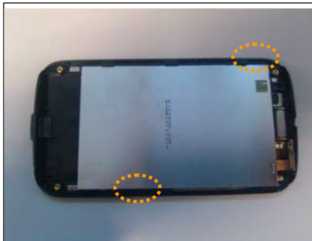
7. Install the LCD. Ensure that the two latches are snapped in place and that the LCD is even.
