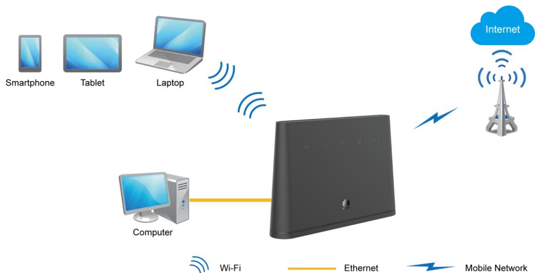
Figure 4-1 Accessing the Internet through a mobile network
