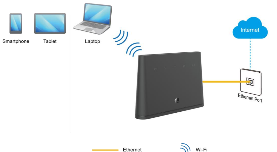
Figure 4-2 Accessing the Internet through an Ethernet network
