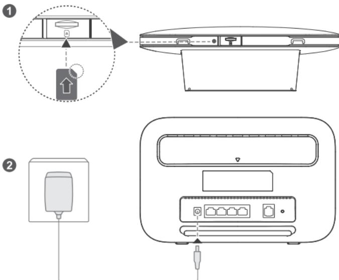
Insert a micro-SIM card into the micro-SIM card slot as shown in the preceding diagram and then connect the power adapter to the B612 router. The router will turn on automatically and search for available mobile networks.
