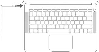
Your MateBook D is pre-installed with an irremovable, rechargeable battery. You can charge your MateBook D with the adapter and USB-C charging cable that comes with it. The battery is sufficiently charged when the charging indicator stays steady white.
