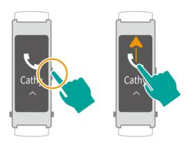
When the headset is in the strap and you don't want to answer the call, touch the screen or press the side button to stop your HUAWEI TalkBand B3 vibrating.
