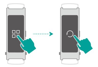
If screen operations can't be performed, press and hold the side button for 10 seconds to force your HUAWEI TalkBand B3 to restart.
