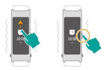
**To snooze a smart alarm:** When an alarm goes off, simply touch the screen of your HUAWEI TalkBand B3 to stop the vibration. Your HUAWEI TalkBand B3 will vibrate again after another 10 minutes. An alarm can be snoozed up to three times.
