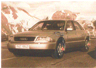
High-temperature tests – driving down a pass, with tire temperatures of far above 100 °C (AUDI)
