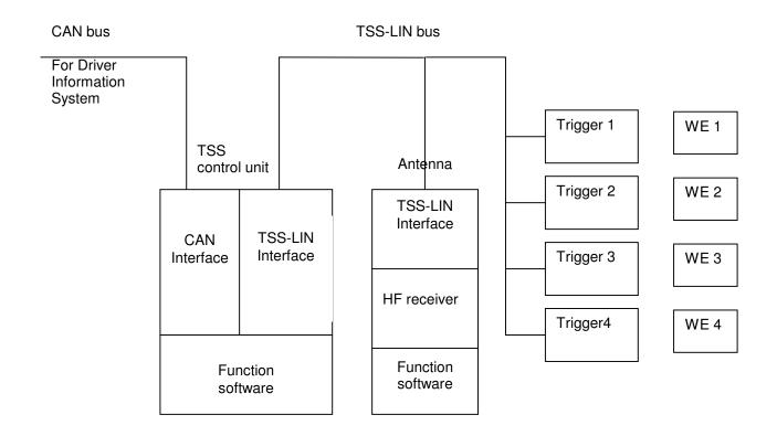
Figure 1: Block diagram, TSS system of the second generation
