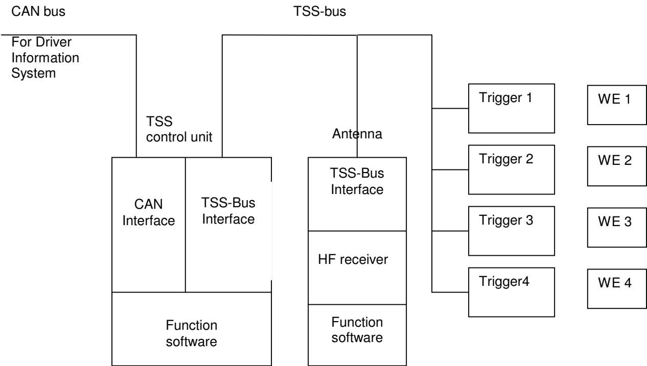
**Figure 1: Block diagram, TSS system of the second generation**
