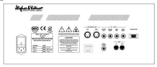
**MAINS IN:** Connect the factory-included mains cord to this socket. Ensure the amp's voltage rating matches your local AC voltage rating before you plug the cord into the wall socket. The mains fuse bracket is located next to this socket (see also Section 8.2). When replacing blown fuses, make sure you use specified replacement fuses only (see 7.0 TECHNICAL SPECIFICATIONS).
