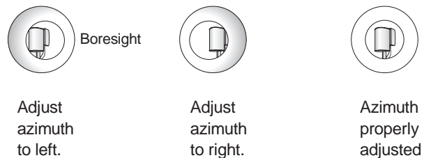
Figure 6-14 Using the boresight to adjust azimuth
