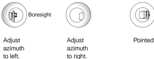
Figure 6-25 Using the boresight to adjust azimuth
