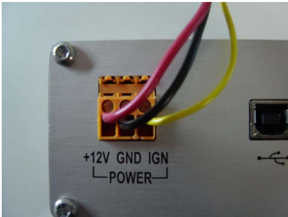
Figure 4 Power Connector with Power Cables Installed
