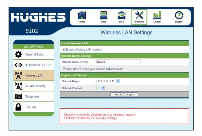
If you have not previously used the terminal's WLAN interface, it has to first be enabled from this page using a computer connected to the terminal using an Ethernet connection. Once WLAN is enabled/configured, TEs can connect to the terminal wirelessly.
