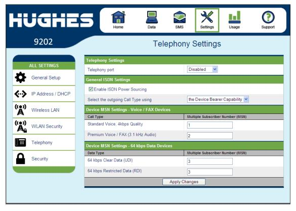
There is also an option under the drop down arrow to set the trigger to use the **MSN** rather than the bearer. If there is a problem using the bearer capability setting, this field can be changed to use the MSN number instead.
