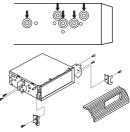
Remove the outer rim around the front panel and the side springs.
