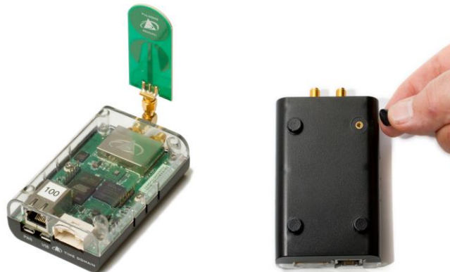
Fig. 4-17: P330 in standard enclosure (left) and view of enclosure bottom showing feet and mounting holes for 4-40 screw
