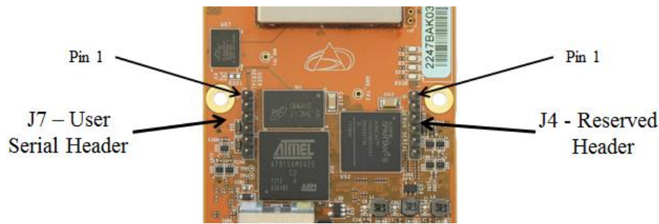
Fig. 4-9: J7 User Serial pinouts
