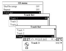
For Audio CD discs, turn the **TUNE dial** from the CD menu to move to the track list, and then press the **MENU button**.
