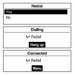
From the steering wheel remote controller, press the **Call** button to display the redial guidance screen, or hold down the button to display the caller log screen.
