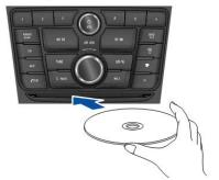
Insert the disc to be played with printed surface facing upward in the disc inserting slot.
