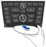
To end play, press the **EJECT** button to take out the disc.
