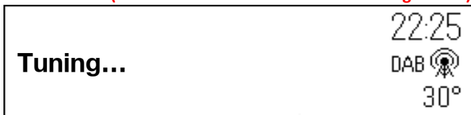
Figure 5.14.2 - tuning screen used when changing ensembles (also known as the intermediate tuning screen)
