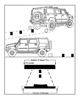
Notice: The spare tire extends farther away from rear of the vehicle than the trailer hitch shown on rear vision camera display. The spare tire could hit an object even though there appears to be enough distance on the display between the trailer hitch and objects behind you causing vehicle or property damage. Do not use this system to judge the distance between the spare tire and objects behind you.
