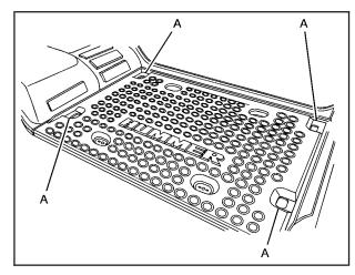
For vehicles with a cargo mat, located under it are four cargo-area floor drains (A) near the sides of the cargo area. These drains should be cleaned periodically to allow water to exit the cargo area.
