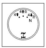
The transfer case dial is located to the right of the instrument panel cluster. Use this switch to shift into and out of the different Full-Time Four-Wheel Drive modes.
