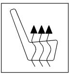
Driver Side RSA Heated Seat Button shown On vehicles with rear outboard heated seats, the buttons used to control this feature are located on the Rear Seat Audio (RSA) panel. ## (Heated Seat): To heat the seat cushion, press the button with the heated seat symbol.
