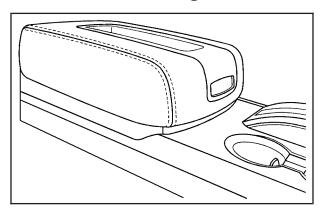
To open the front center console, press the button and lift up.
