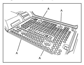
There are four oval shaped openings (A) in the cargo bed that allow access to four tie downs. The tie downs can be used to secure cargo.
