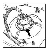
Turn the bulb socket counterclockwise and pull it out of the headlamp assembly.
