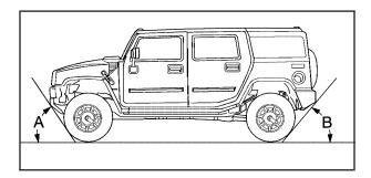
The vehicle has an approximate approach angle (A) of 42° and a departure angle (B) of 37°.
