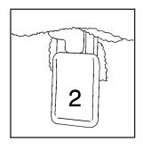
Unlatch the seat from the floor by pulling up on the lever labeled 2, located on the rear of the seat.
