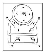
If your vehicle has outside power foldaway mirrors, the controls are located on the driver's door armrest.
