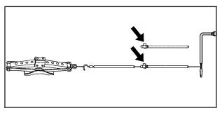
Assemble the jack together with the jack handle and the jack handle extensions, as shown above.
