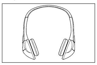
The RSE includes two 2-channel wireless headphones that are dedicated to this system. Channel 1 is dedicated to the DVD player, while Channel 2 is dedicated to RSA selections. These headphones can be used to listen to the radio, CDs, DVDs, MP3s, DVDAs, any auxiliary source connected to A/V jacks, or the auxiliary input jack, if the vehicle has this feature. The wireless headphones have an On/Off button, channel 1/2 switch, and a volume control.
