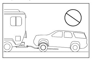
The vehicle cannot be dolly towed. If the vehicle must be towed behind another vehicle, use the dinghy towing procedure explained previously.
