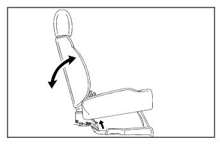
The lever used to operate them is located on the outboard side of the seat(s).
