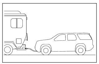
This full-time four-wheel-drive vehicle can be dinghy towed from the front. These vehicles can also be towed by placing them on a platform trailer with all four wheels off the ground. These vehicles cannot be towed using a dolly.
