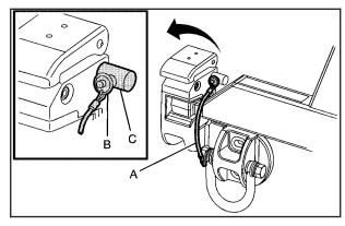
Press the button on the pin (B), which is attached to the cable (A), to remove the pin from the latch nut (C).
