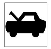
Pull the handle with this symbol on it. It is located inside the vehicle to the lower left of the steering column.
