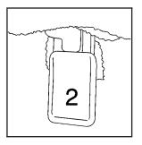
Pull up on the release lever labeled 2, at the rear of the seat, to unlatch the rear of the seat from the floor, and lift the rear of the seat up from the floor.
