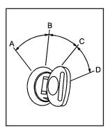
The ignition switch has four different positions.
