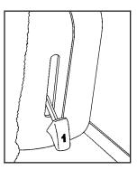
Pull up on the release lever labeled 1 and then pull up on the seatback until the seatback locks into the upright position.
