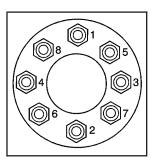
15. Tighten the nuts firmly in a crisscross sequence as shown by turning the wheel wrench with the wheel wrench extender clockwise.
