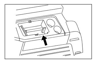
Return the storage tray to its original location by pushing down on the finger depression.
