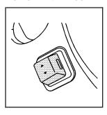
For vehicles with the power tilt wheel control it is located on the left side of the steering column.
