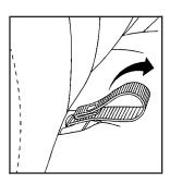
Pull up on the strap loop located at the rear of the seat cushion and pull the seat cushion up and fold it forward. Notice: Folding a rear seat with the safety belts still fastened may cause damage to the seat or the safety belts. Always unbuckle the safety belts and return them to their normal stowed position before folding a rear seat.
