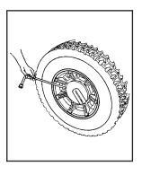
To remove the center cap, place the flat end of the wheel wrench in the slot on the wheel and carefully pry the center cap out.
