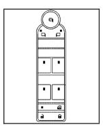
A power window switch is located on the armrest of each side door. The switches operate while the ignition is in ON/RUN or ACC/ACCESSORY or while Retained Accessory Power (RAP) is active. See *Retained Accessory Power (RAP) on page 2-29.*
