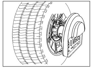
Slide the license plate holder onto the spare or flat tire. Secure it from the back of the tire carrier with the wing nut.
