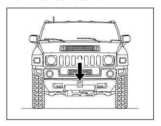
This vehicle is equipped with a front mounted receiver.
