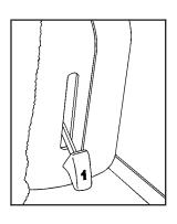
Pull up on the release lever labeled 1 and then pull up on the seatback until the seatback locks into the upright position.
