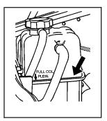
The coolant surge tank is located in the engine compartment on the passenger side of the vehicle. See Engine Compartment Overview on page 5-14 for more information on location.
