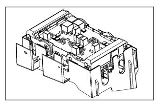
The underhood fuse block in the engine compartment is located on the driver side of the vehicle near the battery. Lift the cover for access to the fuse/relay block.
