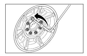
Turn the wheel wrench counterclockwise to loosen the wheel nuts. Do not remove them yet.
