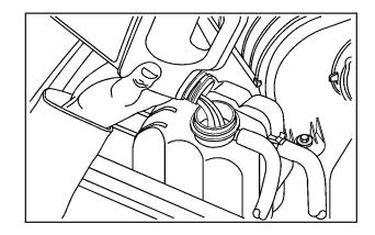
Fill the coolant surge tank with the proper mixture, to the FULL COLD mark.
