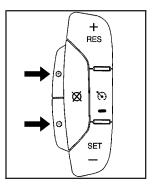
The vehicle has Driver Shift Control (DSC). DSC controls the transmission and vehicle speed while driving down hill or towing a trailer by allowing you to select a desired range of gears.
