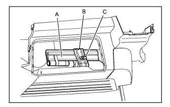
Turn the retainer nut (C) counterclockwise. Remove the tool bag (A) and the two wheel blocks (B) from the storage area. Open the tool bag. The following tools needed to remove the spare tire and flat tire are inside the tool bag:
