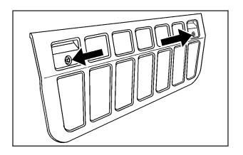
3. Press either one of the two power Midgate latch release buttons. The Midgate will move slightly forward from its closed position. The latch release buttons operate while the ignition is in ON/RUN, ACC/ACCESSORY, in RAP mode, or up to 10 minutes after removing the key. If necessary, press the global express-down button to reactivate the release buttons for an additional 10 minutes.
