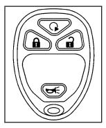
**Q** (Remote Vehicle Start): Press to start the engine from outside the vehicle using the RKE transmitter. See *Remote Vehicle Start on page 2-7* for additional information.
