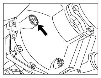
When the differential is cold, the proper level is from about 1/4 inch (6 mm) to about 3/8 inch (10 mm) below the filler plug hole.
