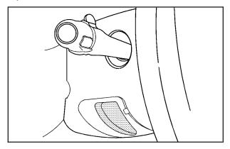
The tilt lever is located on the left side of the steering column.
