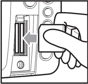
Inserting an SD Card
