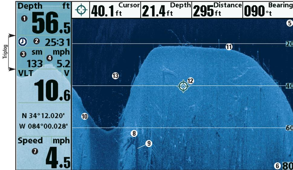
**7 Speed** - If a GPS Receiver or Temp/Speed accessory is connected, the Fishing System can display the speed of the boat and can keep a Triplog of nautical or statute miles traveled.
