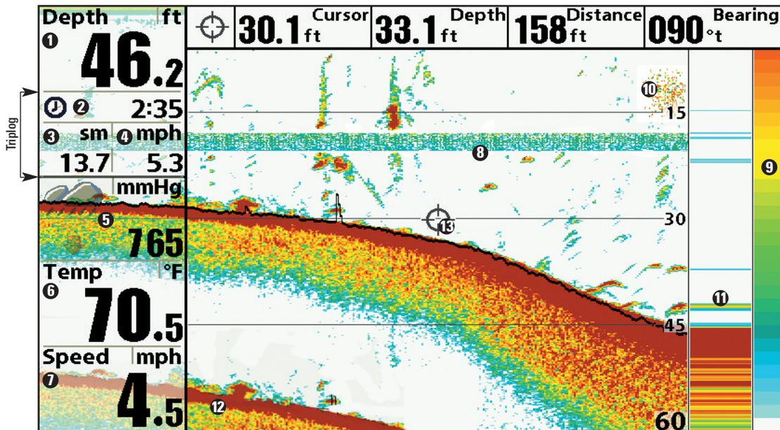
**8** Thermoclines - Layers of water with different temperatures that appear at different depths and different times of the year. A thermocline typically appears as a continuous band of many colors moving across the display at the same depth.
