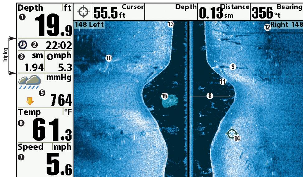
**8** **Water column** - Shows the relative depth of the water under the boat at a given time. Variations in the width of the water column show variations in the distance to the bottom as the boat passes over.
