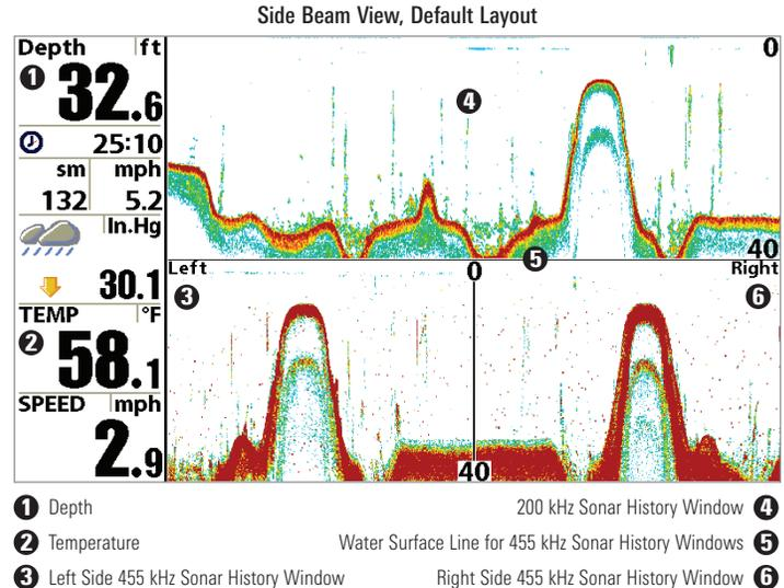
**Classic layout:** The top portion of the display presents a historical log of sonar returns from the 200 kHz down-looking sonar beam. New information in the down beam panel scrolls from right to left. The bottom portion of the display presents a historical log of sonar returns from the 455 kHz right- and left-looking sonar beams. New information appears at the top and scrolls down the display.
