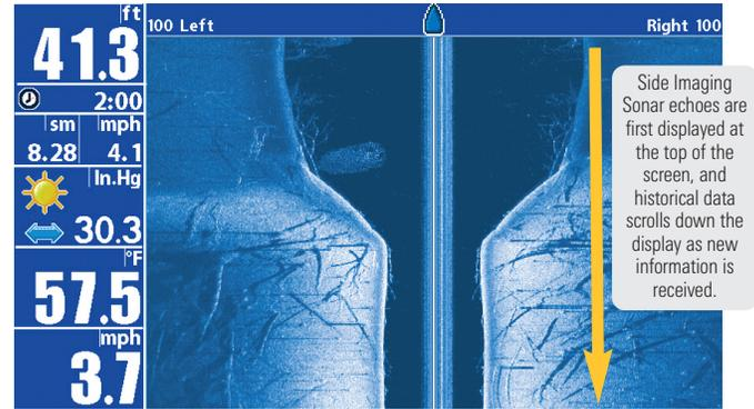
Side Imaging Sonar echoes are first displayed at the top of the screen, and historical data scrolls down the display as new information is received.
