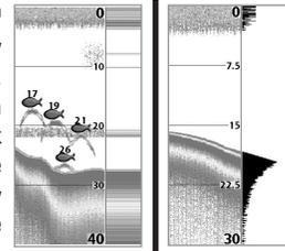
The **Wide RTS Window™** indicates the sonar intensity through the use of a bar graph. The length of the plotted return provides an indication of whether the return is weak or strong. The depth of the sonar return is indicated by the vertical placement of the return on the display depth scale.
