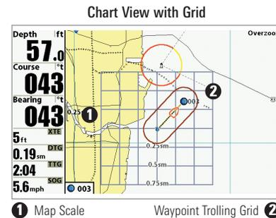
**Add a Trolling Grid:** From the Waypoints submenu, select Grid, and press the RIGHT Cursor key to display the saved waypoints list. Select a waypoint and press the RIGHT Cursor key. The grid can also be rotated to any heading by adjusting the Grid Rotation setting on the Navigation Menu Tab.
