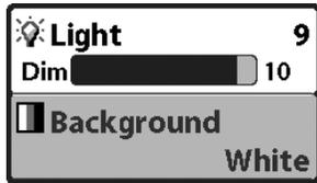
**Adjust the Backlight or the Display Background Color:** Press the POWER/LIGHT key to access the Light and Background submenu. Use the 4-WAY Cursor Control key to select Light or Background, and then use the LEFT or RIGHT Cursor key to change the settings. Press EXIT to exit the Light and Background submenu.
