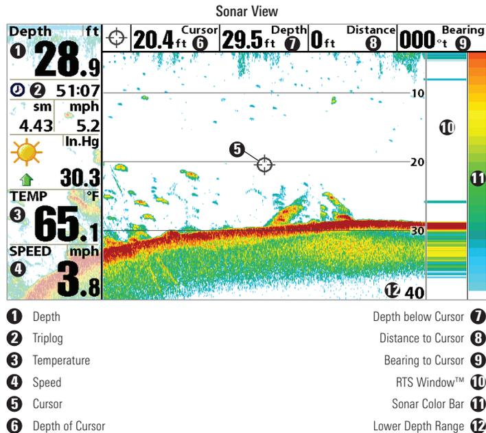
**NOTE:** If the Depth number is flashing, it means that the unit is having trouble locating the bottom. This usually happens if the water is too deep, the transducer is out of the water, the boat is moving too fast, or for any other reason that the unit can't accurately receive continuous data.
