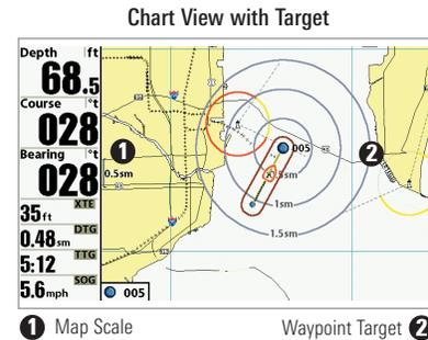
**Add a Waypoint Target:** From the Waypoints submenu, select Target, and press the RIGHT Cursor key to display the saved waypoints list. Select a waypoint and press the RIGHT Cursor key.
