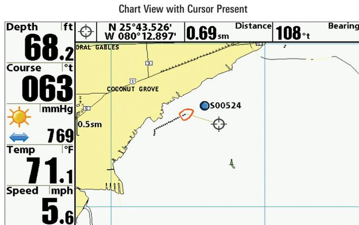
**Zooming:** Press the Plus (+) key to Zoom In and the Minus (-) key to Zoom Out to see the cartography at different magnification levels. The zoom level is indicated on the left side of the display. If you zoom in beyond the available chart data, the display will go into Overzoom mode whereby the last available chart data is amplified to reflect the level selected. If you zoom in so far that no cartography is available, a lat/long grid will be drawn instead.
