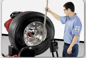
The standard hook tool is used to mount and demount tubed and super single tires or more difficult-to-handle wheel assemblies.
