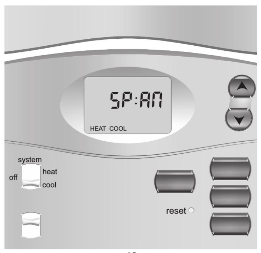
3. Span setting mode – allows you to adjust the system ON/OFF cycle rate. The default setting is 2 (the system cycles ON or OFF when the temperature is within 1° F (0.5° C) above and below the set temperature.) The span setting can be adjusted if your system is cycling too fast or too slowly.
