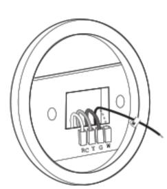
(If the terminals are not labeled, contact a qualified HVAC technician.)
