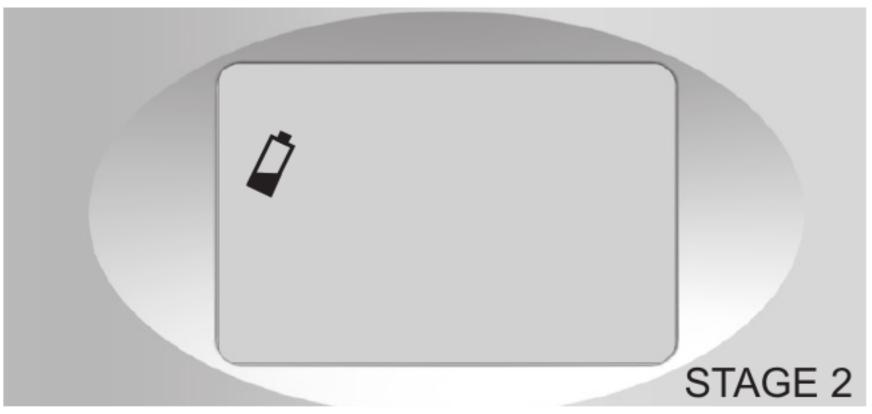
Low battery warning – indicates two stages of battery power shortage.
