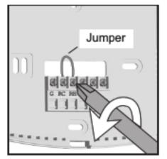
Note: A jumper wire has been provided, connecting the RC and RH terminals for systems that do not provide both an RH and RC wire. If you have both an RH and RC wire, remove this jumper. If you do not have both an RH and RC wire, leave the jumper in
