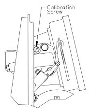
Replace the cap screw (old style only). Deliver about 1/2 gallon through the meter before resetting to zero and retesting. Allow a ten second drain period each time the test measure is emptied to assure accurate measure. Adjust and retest until register is zeroed at desired flow.
