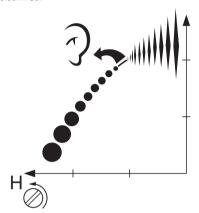
You have now run the machine at settings of H =±0, H=+1/4, H=+1/2 relative to the basic settings. At full throttle the engine has sounded different for each setting. The H-jet is correctly adjusted when the machine burbles a little. If the machine "screams" then the machine is set too lean. If the muffler emits a lot of smoke and the machine burbles a lot then the setting is too rich. Turn the H-jet clockwise until the setting sounds right
