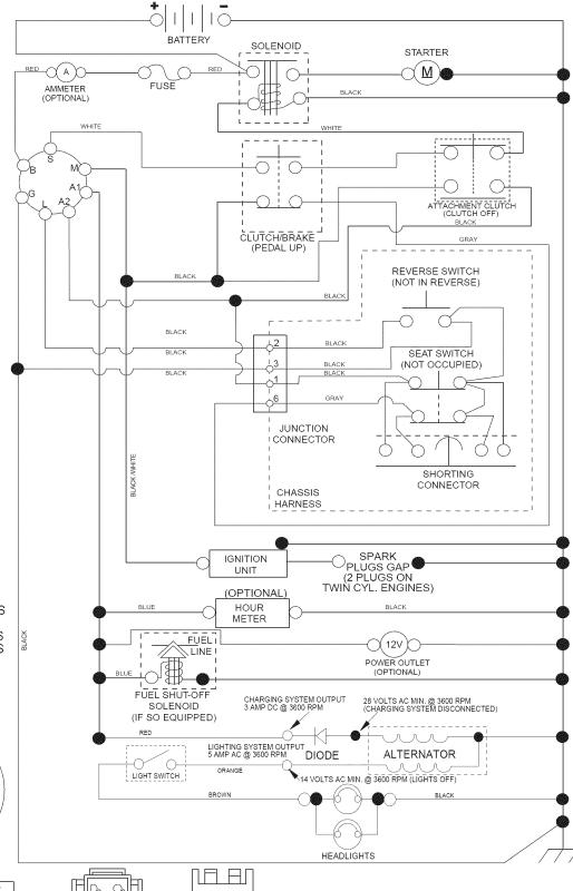
NOTE YOUR TRACTOR IS EQUIPPED WITH A SPECIAL ALTERNATOR SYSTEM. THE LIGHTS ARE NOT CONNECTED TO THE BATTERY, BUT HAVE THEIR OWN ELECTRICAL SOURCE. BECAUSE OF THIS, THE BRIGHTNESS OF THE LIGHTS WILL CHANGE WITH ENGINE SPEED. AT IDLE THE LIGHTS WILL DIM. AS THE ENGINE IS SPEEDED UP, THE LIGHTS WILL BECOMÉ THEIR BRIGHTEST.
