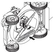
5 The bolt should be tightened with a torque of 35-40 ft. lbs. / 47-54 Nm. 6 Verify the spark plug wire is disconnected from the engine.
