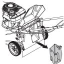
2 Close the back shield to allow the machine to discharge material to the left of the machine while cutting.
