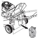
2 Lift the back shield and place the grass catcher frame hooks onto the grass bag brackets.
