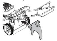
3 Close the back shield to allow the machine to discharge material to the left of the machine while cutting
