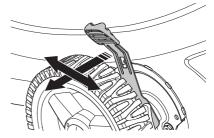
· The adjuster lever is spring loaded.
