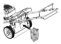
3 Allow the back shield to close and ensure the back shield is firmly shut against the mulch plug.
