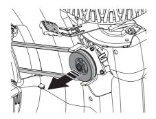
Pull out the belt and thread it over the adapter.
