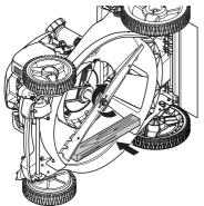
5 The bolt should be tightened with a torque of 35-40 ft. lbs. / 47-54 Nm.
