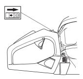
Start the engine and make sure the engine stops when you move the stop switch to the stop setting.
