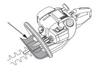
Check that the hand guard is fitted correctly.
