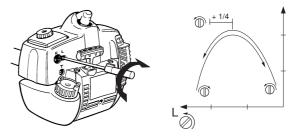
**CAUTION!** If the blades move while the engine is idling the T screw should be turned anti-clockwise until they stop.
