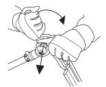
5 Fold down the cutting unit against the shaft.
