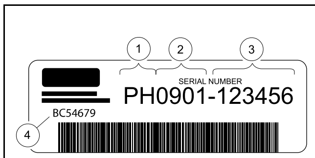
1400 Figure 6 Serial Number Decal with the Vehicle Build Code
