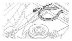
4 Slide in the cutting deck and put the guide plugs in the grooves on the equipment frame, one on each side.
