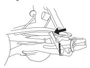
3 Place the belt and the cable in such a way to prevent them from being crushed.
