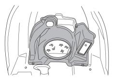
A clogged air intake grille, air duct or cooling air intake impairs the cooling of the engine, which may result in engine damage.
