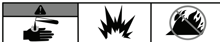
Battery acid is corrosive, explosive and flammable
