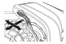
· The adjuster lever is spring loaded.
