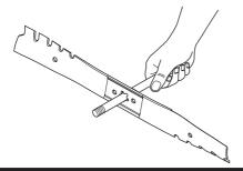
IMPORTANT! The blades should be balanced after sharpening. We do not recommend sharpening blade. Sharpening and balancing the blade should be conducted by an authorized service workshop.
