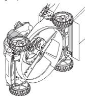
Use a wood block between blade and mower housing to prevent blade from turning when removing blade holt
