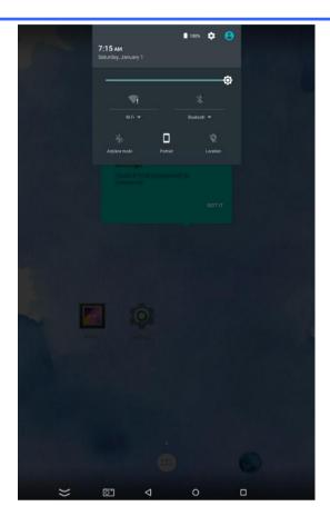
Information regarding the current state of the tablet and its latest notifications will appear here. The quick setting menu allows for convenient access to change the configuration of a handful of selected settings (e.g. Screen brightness, WiFi Access and Airplane Mode).
