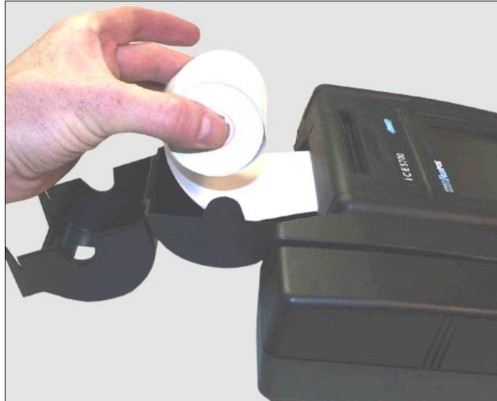
Figure 3-2. ICE 5700 printer paper installation
