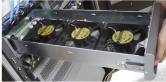
Figure 3-12 Installing the FAN
