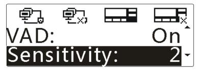
**Step 5** Press the **OK** key, and then press the **Up/Down** key to set the sensitivity level, as shown below.
