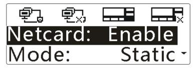
**Step 4** Press the **OK** key to select "Netcard", and then press the **Up/Down** key to highlight "Enable" or "Disable".
