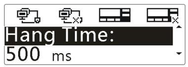
Step 5 Press the OK key, and then press the Up/Down key to set the time, as shown below.
