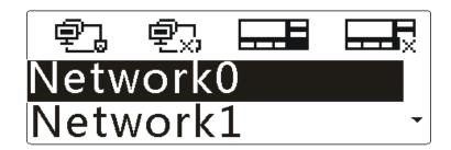
**Step 3** Press the **Up/Down** key to highlight "Network0" or "Network1", and then press the **OK** key to enter the menu.
