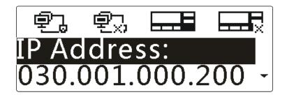
**Step 7** Press the **Up/Down** key to highlight "IP Address", and then press the **OK** key.
