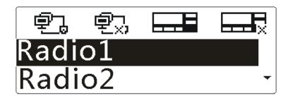
**Step 3** Press the **Up/Down** key to highlight "Radio1" or "Radio2", and then press the **OK** key to enter the menu.
