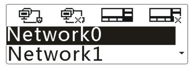
**Step 3** Press the **Up/Down** key to highlight "Network0" or "Network1", and then press the **OK** key to enter the menu.
