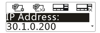
**Step 4** Press the **Up/Down** key to view the local IP address, subnet mask, default gateway and MAC address.
