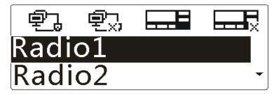
**Step 3** Press the **Up/Down** key to highlight "Radio1" or "Radio2", and then press the **OK** key to enter the menu.
