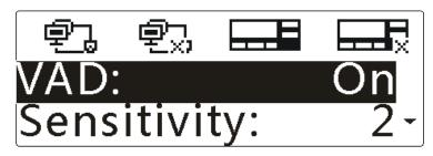
Step 4 Press the OK key to select "VAD", and then press the Up/Down key to highlight "On" or "Off".
