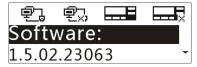
**Step 4** Press the **Up/Down** key to view the version of software and hardware.
