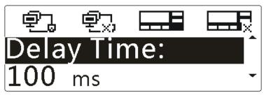
**Step 5** Press the **OK** key, and then press the **Up/Down** key to set the time, as shown below.
