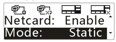
**Step 5** Press the **OK** key, and then press the **Up/Down** key to highlight "Dhcp", as shown below.
