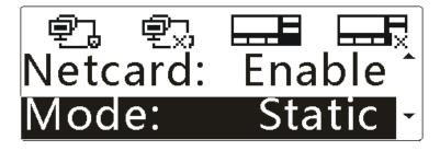
**Step 5** Press the **OK** key, and then press the **Up/Down** key to highlight "Static", as shown below.
