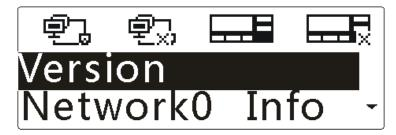
**Step 3** Press the **Up/Down** key to highlight "Network0 Info" or "Network1 Info", and then press the **OK** key to enter the menu.
