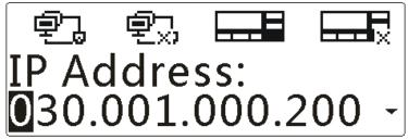
**Step 8** Press the **Up/Down** key to change the value, and then press the **OK** key to confirm the value.
