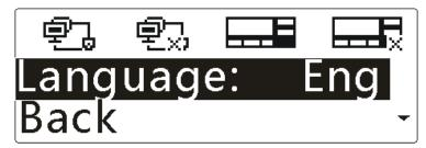
Step 3 Press the OK key, and then press the Up/Down key to highlight "中文" or "Eng", as shown below.
