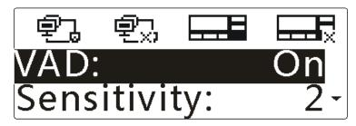
**Step 4** Press the **Down** key to highlight "Sensitivity", as shown below.
