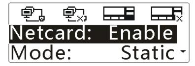
Step 4 Press the **Down** key to highlight "Mode", as shown below.
