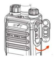
**Step 2** Align the accessory (such as an audio accessory, or a programming cable) plug with the accessory connector.
